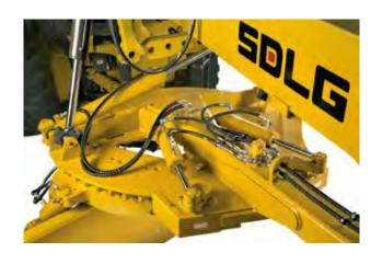
■ The SDLG dual gear Circle Drive System uses direct acting hydraulic power and two hardened drive pinions for exceptional turning and holding capability under full load.
